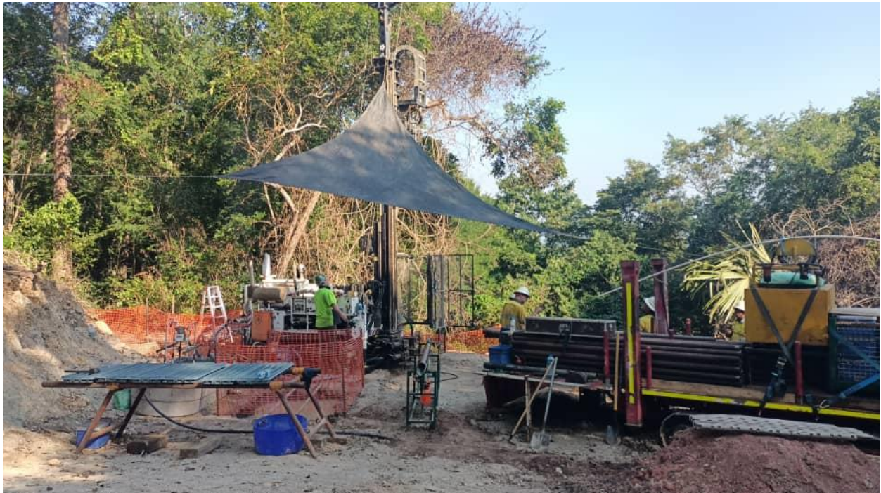
Figure 1: Diamond drilling operations underway collaring EMDD002 at the Ira Miri discovery as part of the first ever modern minerals exploration campaign in Timor-Leste
