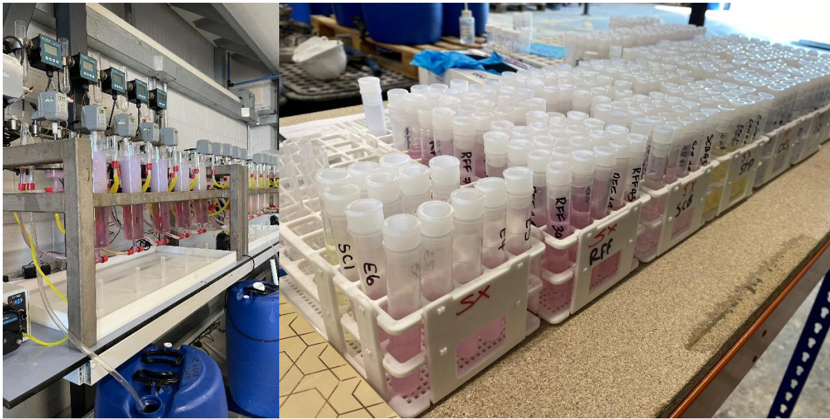
Figure 1: Continuous rare earth separation test work (left), and refinery Solvent Extraction test work samples used to develop Ionic Technologies' flowsheet and process model for U.S. Refinery (right) based on the Makuutu Project MREC.
