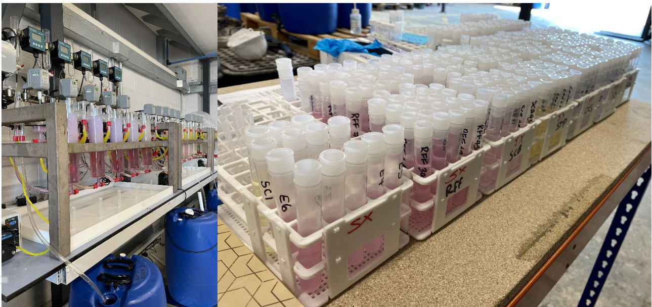
Figure 1: Continuous heavy rare earth separation test work (left), and refinery SX test work samples used to develop Ionic Technologies flowsheet and process model for US Refinery (right).
