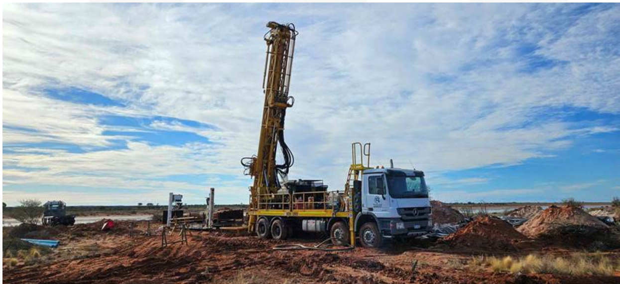
Plate 1 – Diamond drill rig set up on 25FNDD011
