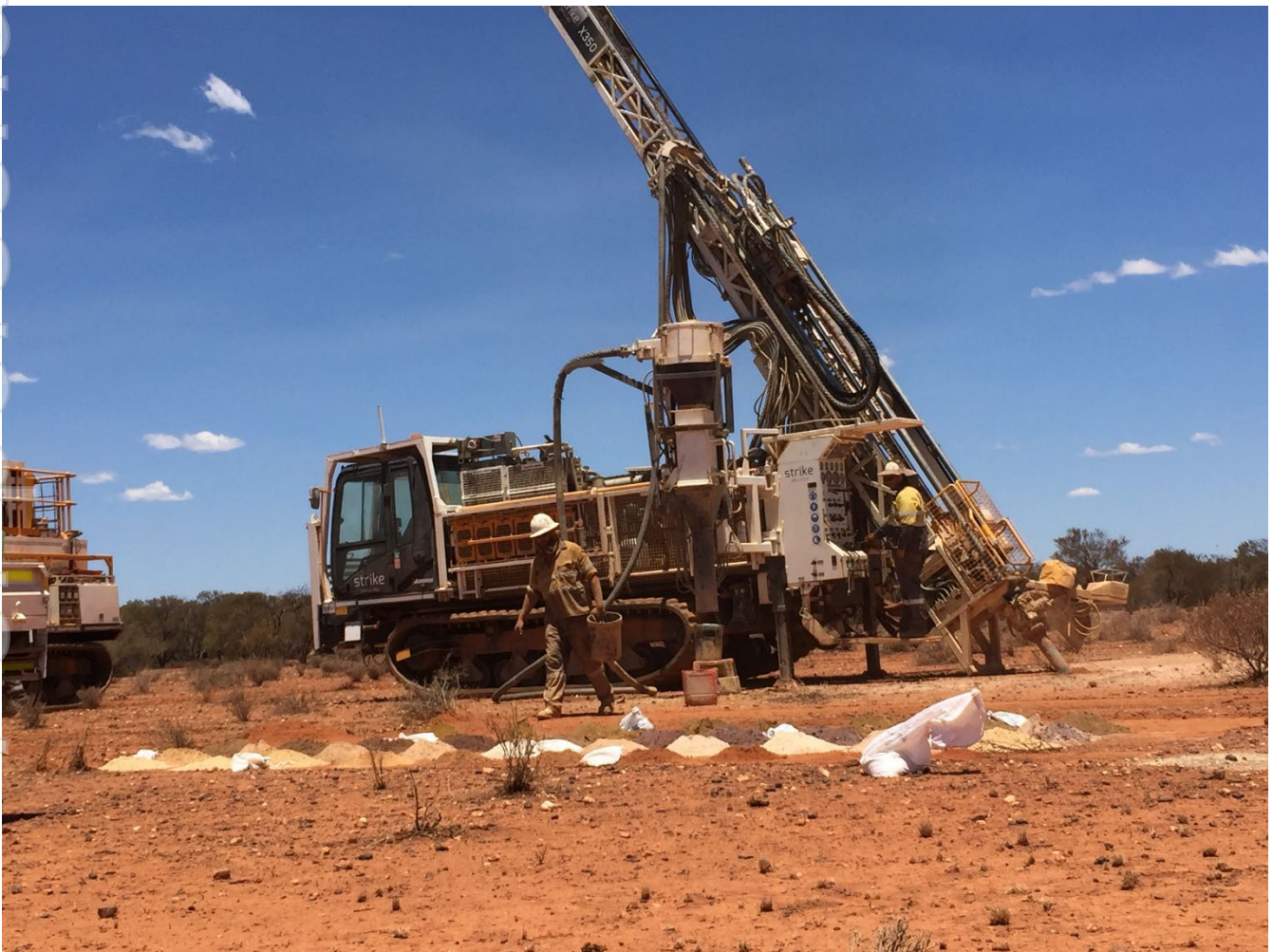
Photo: Multi-purpose Air-core and Reverse Circulation Rig at Yundamindra
