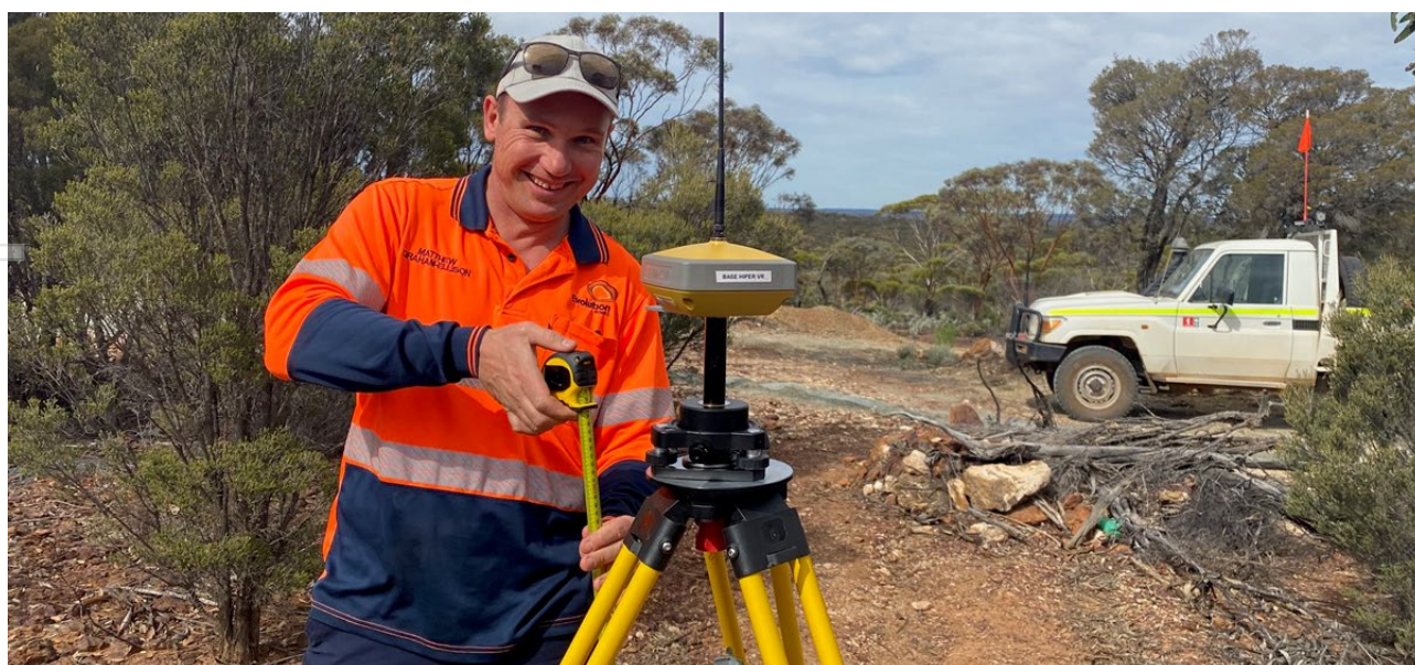
Photo 3: Matthew setting up base station. Photo: 15 June 2025.
