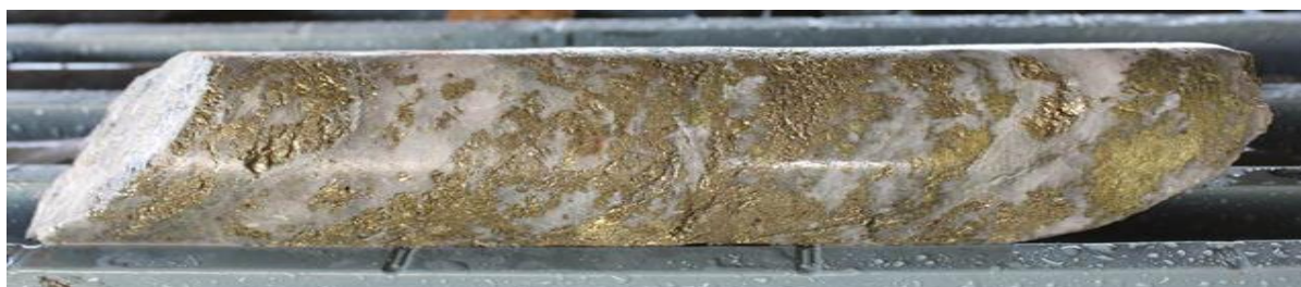
Figure 2 – The main quartz-carbonate-pyrite-chalcopyrite vein with strong sericite-chlorite selvages of the Displaced Lode mineralisation in DTDD056 (143.5 – 143.9m).
