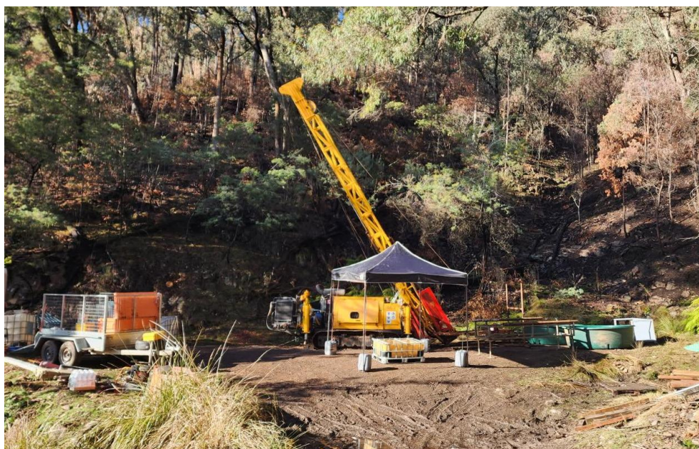
Figure 1. Photograph taken 17 June 2025 showing the diamond drilling rig drilling new hole AMD009 at the Happy Valley Prospect, Myrtleford Project, Victoria.
