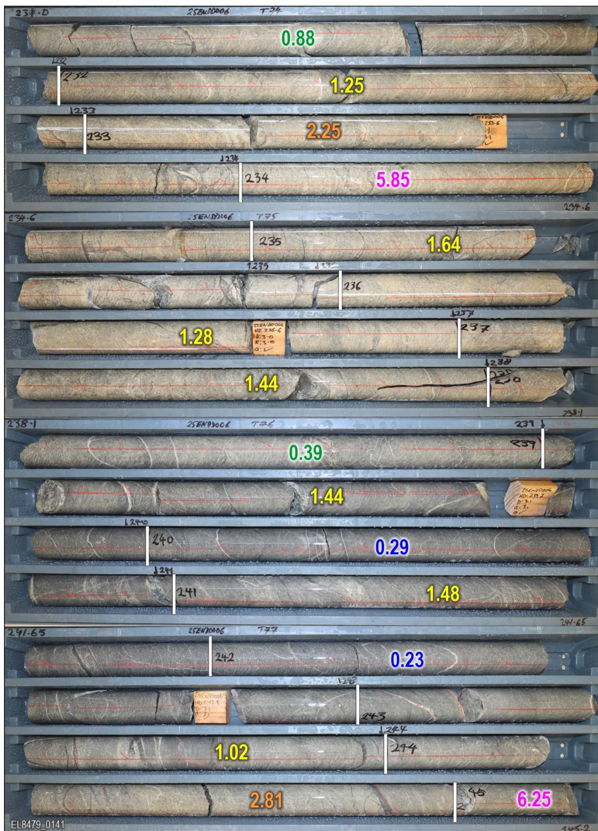
Photo 6 (continued from previous page). Core tray photos of 25ENDD006 interval 35.5m @ 1.94g/t Au from 210.5m incl. 9.7m @ 3.18g/t Au from 210.5m. Distinctive paler coloured zones (silica-sericite altered) typically host better grades (although not exclusively) and are interpreted to have overprinted the darker coloured zones (propylitic/chlorite altered). The numbers superimposed on the core are the reported gold assay grades over each respective sample interval.
