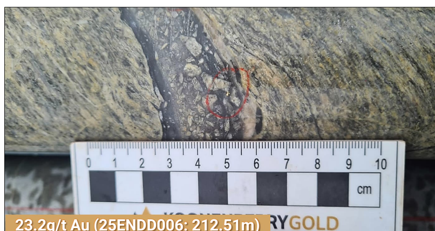
Photo 2. Sample photo of 25ENDD006 from 212.4-212.7m @ 23.2g/t Au with visible gold circled in red associated with Fe-Carbonate quartz-pyrite-arsenian pyrite vein breccia within granite host rock.
