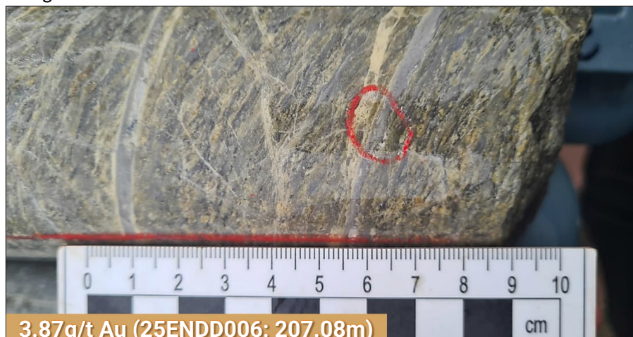
Photo 1. Sample photo of 25ENDD006 from 207-207.3m @ 3.87g/t Au with visible gold circled in red in a quartz-pyrite vein within moderately phyllic altered granite host rock.
