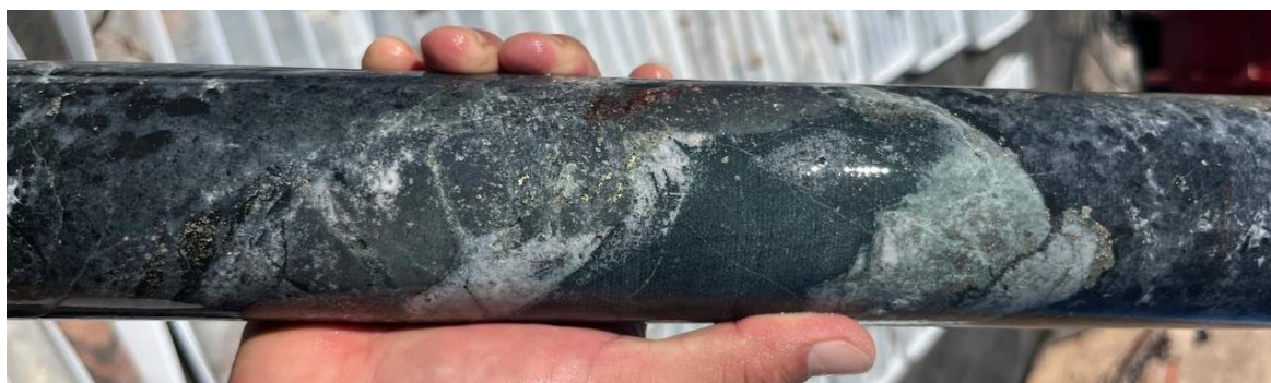
Figure 1: CAP-001-2025 drill core from 184.20 to 184.75 metres displaying tourmaline/specularite breccia with chalcopyrite mineralisation hosted in diorite intrusive. Visually estimated grade 0.5% Cu 1 . Assays are due for release in July / August 2025.
