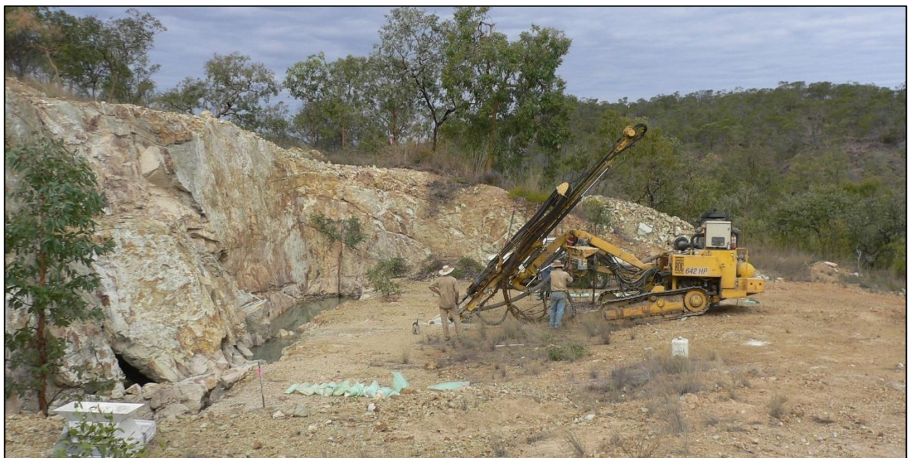
Figure 2: Shallow airtrack drilling beneath the 1991 trial pit at Francis Creek (from CR40465, 2005).
