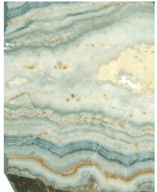
Figure 6: left: Crustiform, colloform quartz-adularia veining (Francis Creek, Sybil), right: Crustiform, colloform quartz-adularia veining (Sonia, Pajingo).
