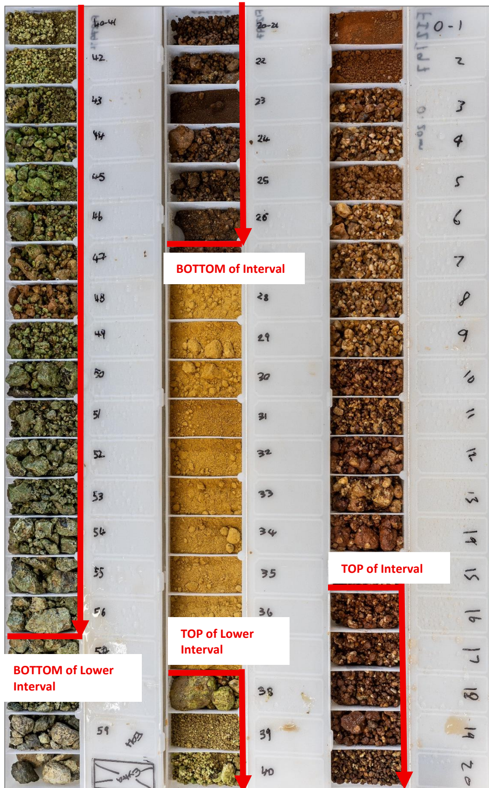
Figure 1: F12797 chip tray photo with scandium intervals highlighted - 11m @ 357 ppm Sc (548ppm Sc Oxide) from 16m including 6m @ 510ppm Sc (782ppm Sc Oxide), 7m @ 176ppm Sc (270ppm Sc Oxide) from 38m and 8m @ 103ppm Sc (158ppm Sc Oxide) from 49 metres. Each compartment in chip tray represents a 1 – metre downhole interval.
