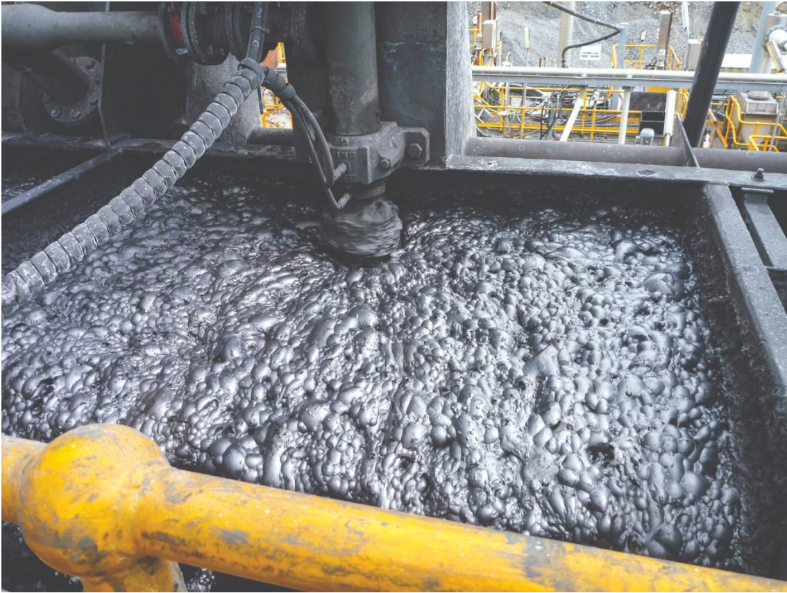
Figure 1: Mineral Hill flotation processing.
