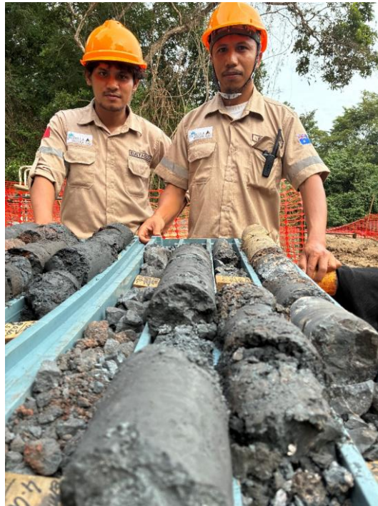
Figure 1: Estrella Geophysicist Eustaquio Amaral and Geologist Gregorio Pereira looking over the massive manganese oxides intersected in the start of diamond drillhole EMDD002. Visual estimates are shown in Table 1.
