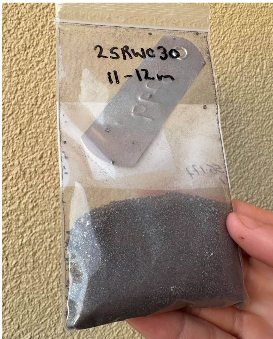
Photo 1 – Exceptional HMC Assay sample from Drill hole 25RW030 returning 55.7% HM from 11-12m.
