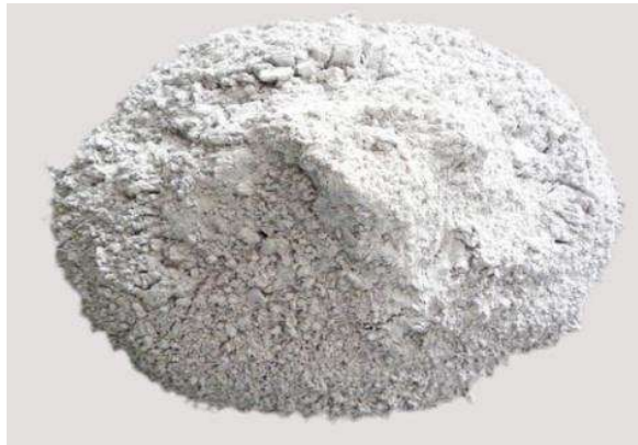
Ground granulated blast furnace slag (GGBFS / Slag) – steel manufacturing by-product
