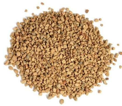
Calcined clay – naturally occurring kaolinite heated to >600°C
