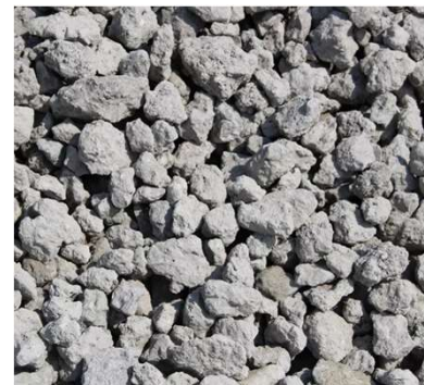
Recycled concrete – processed following end of life
