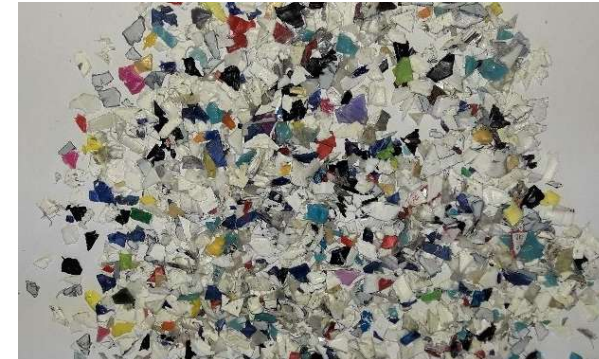
2025: Front-end firing project to introduce hard-to-recycle plastic waste & wood into front end of kiln ~70-80% coal substitution target
