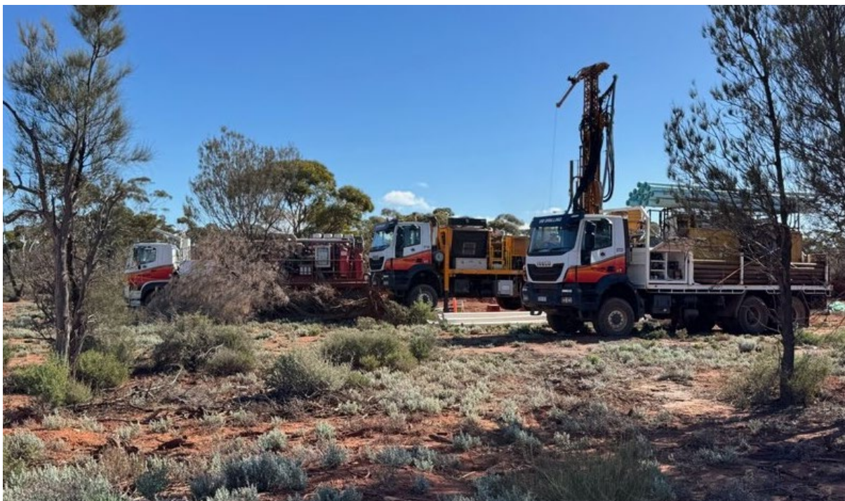
Figure 3: Second RC Drill Rig on site completing pump test holes supporting hydrogeological studies
