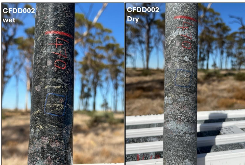
Figure 8: Photo of Centre Forest diamond core within the reported CFDD002 intersection at 470m. The weakly mineralised copper-gold zone is comprised of an interpreted mineral suite of quartz - biotite - amphibole- garnet - cordierite- chalcopyrite - pyrrhotite and pyrite.
