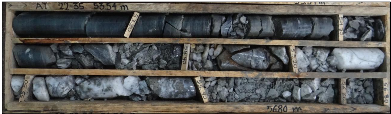
Photo 7. Mineralized intersect in Hole AT-22-35 showing a wide vein zone with well developed vein textures in quartz and zone of semi-massive sulphides. See details in text for this interval.
