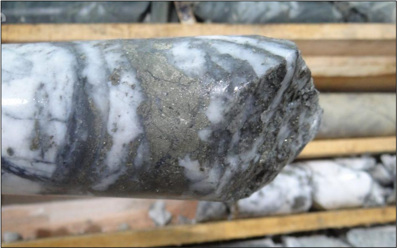
Photo 3. Coarse sulphides (pyrite, sphalerite, galena) with acanthite in quartz in drill core (AT-21-05).
