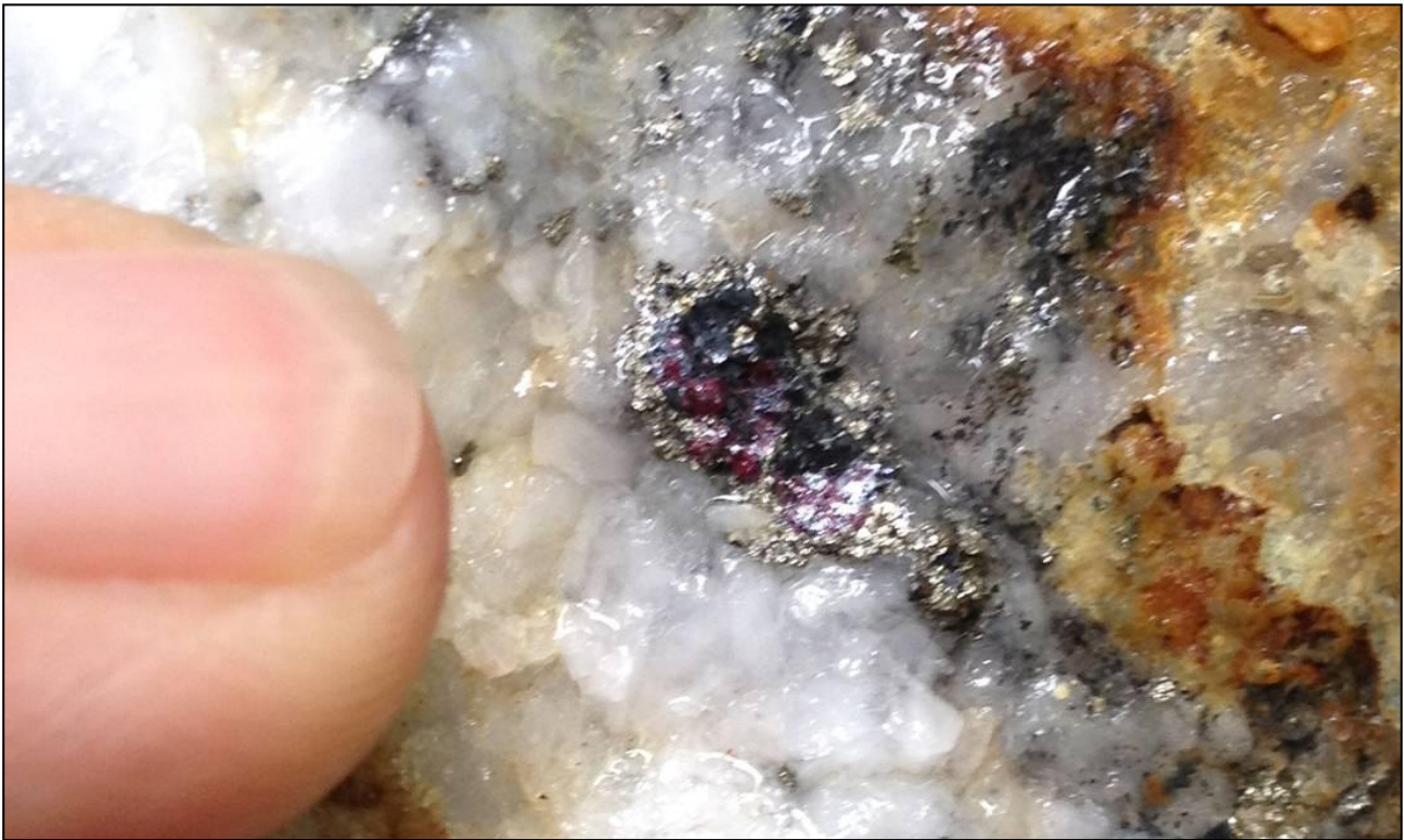
Photo 1. Coarse grained pyrrargyrite enclosed in pyrite and silver sulphosalts in quartz gangue. Veta Grande East.
