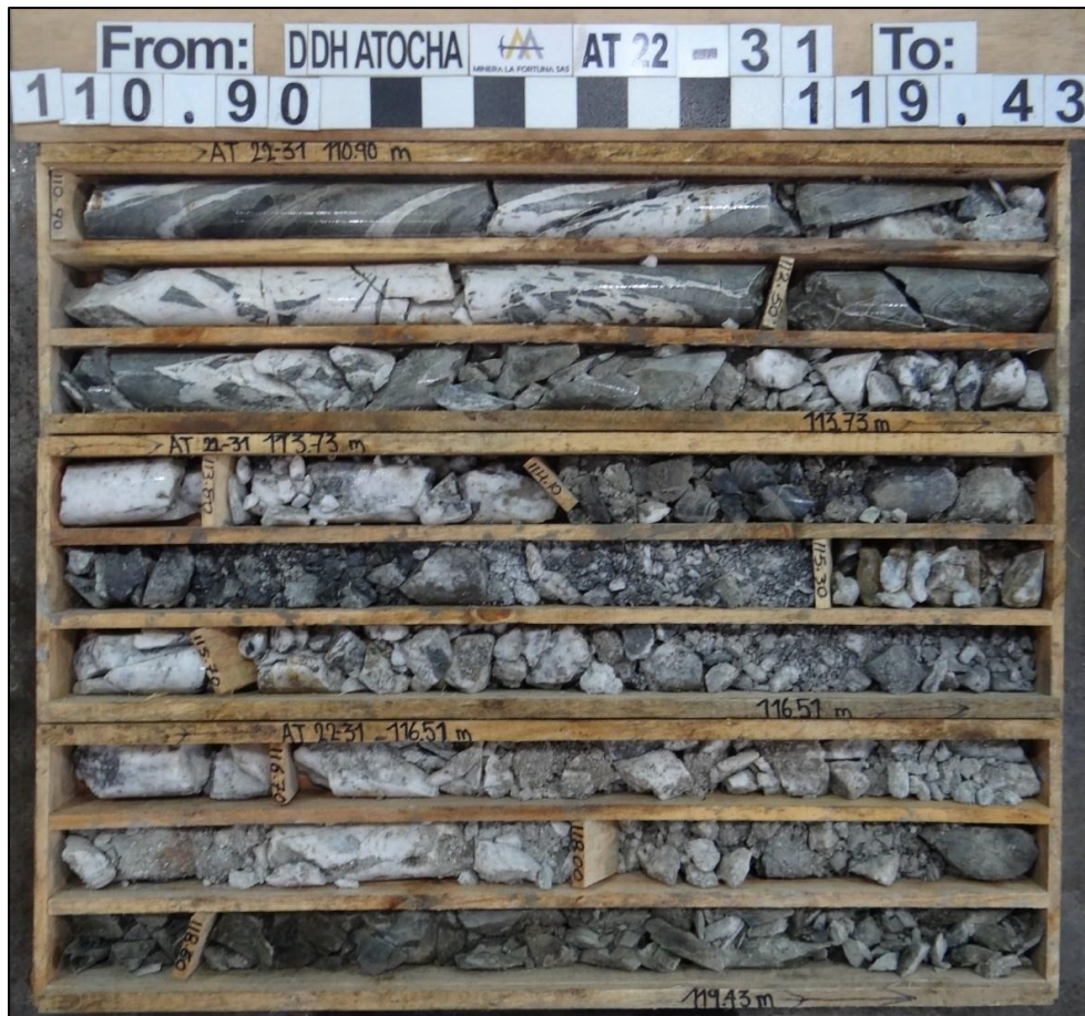
Photo 6. Wide (>7m) mineralized vein zone in hole AT-22-31 from 110.90 to 118.50m.
