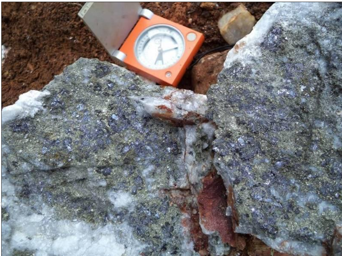
Photo 2. Coarse sulphides (pyrite, sphalerite, galena) in quartz matrix (S2b)
