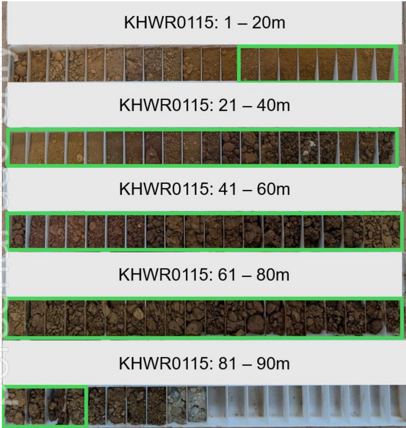
Figure 4 – KHW0115 RC chip trays with significant intercept highlighted (72m at 0.92% Ni, 0.06% Co and 22.7ppm Sc, from 12m downhole)
