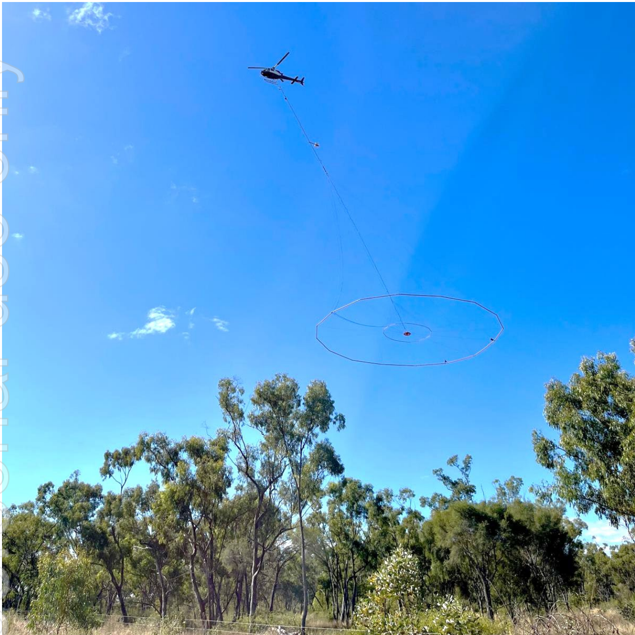
Figure 1: Helicopter-borne VTEM survey in action.
