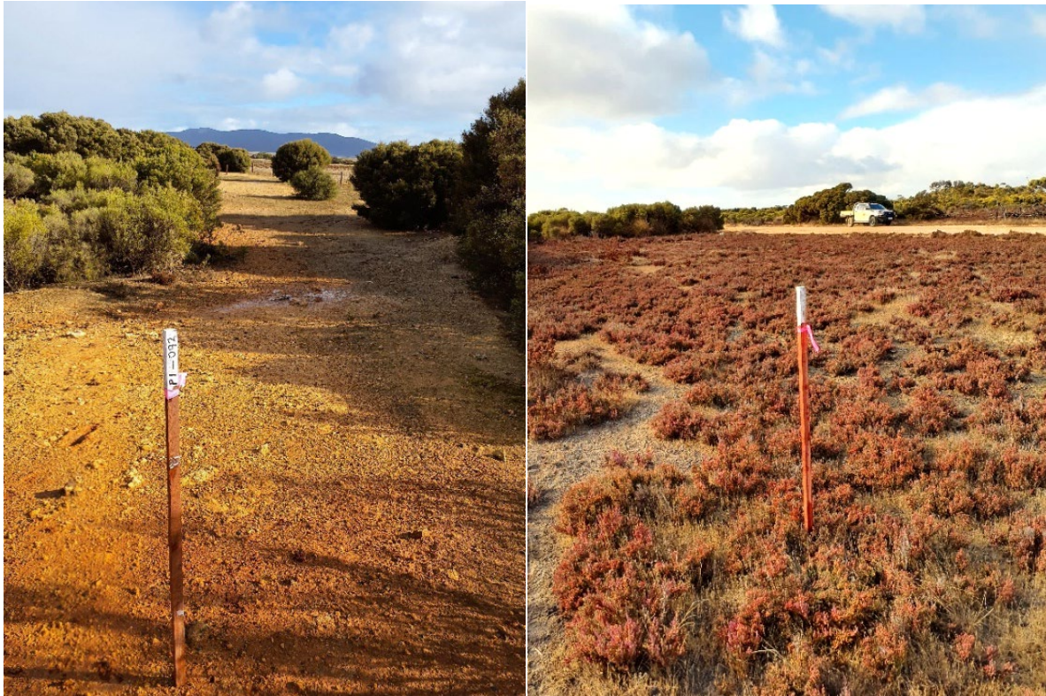
Figure 1: Collar location pegging at Cummins Uranium Project
