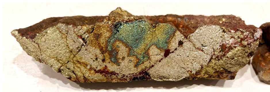
Figure 3c. Photograph: approximately 5cm length of broken core displaying predominantly sulphide minerals. Specimen from 160.6m drill depth in hole D28-DDH4
