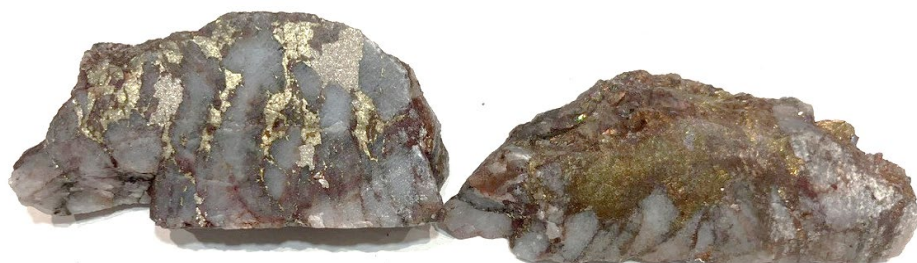
Figure 3b. Photograph: approximately 10cm length of broken core displaying the Cu-Mo hosting sulphide minerals within a quartz vein. Specimen from 160.16m drill depth in hole D28-DDH4
