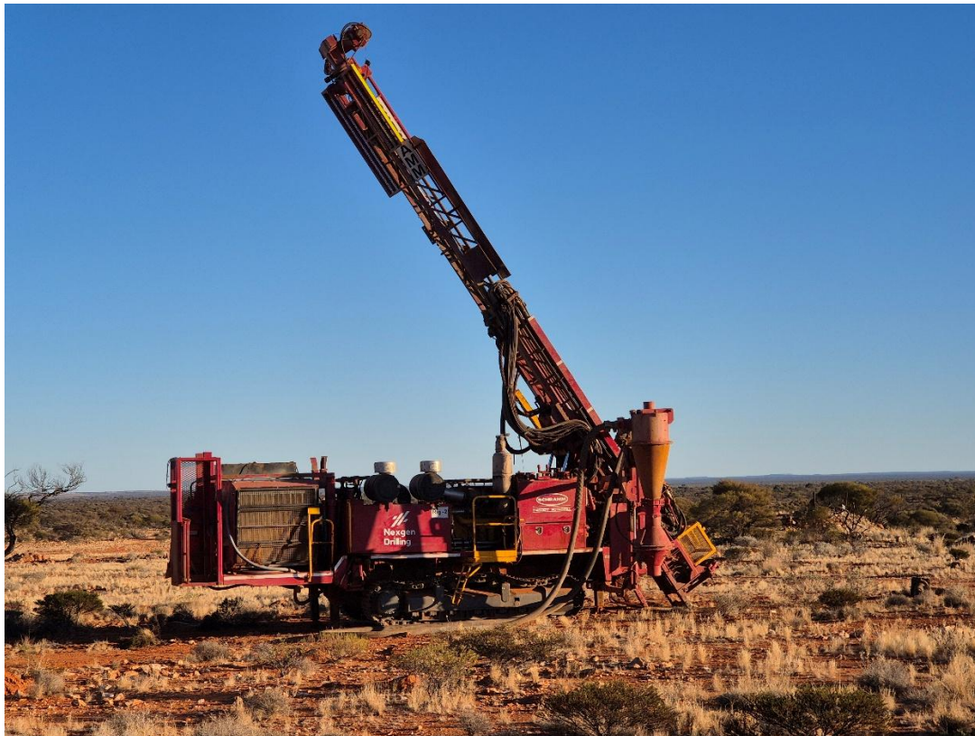
Figure 1: RC drill rig operating at Yandal West, testing high-priority
