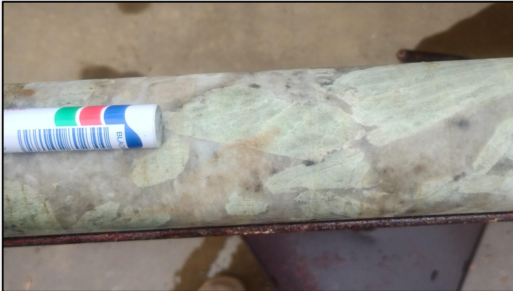
Coarse-grained spodumene in drill core from CLMDD001 @ 147.8m (2.69% Li 2 O)
