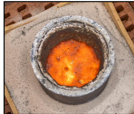
CONVERSION VESSEL COOLING FOLLOWING THE TEST & FERRONIBIUM SAMPLE
