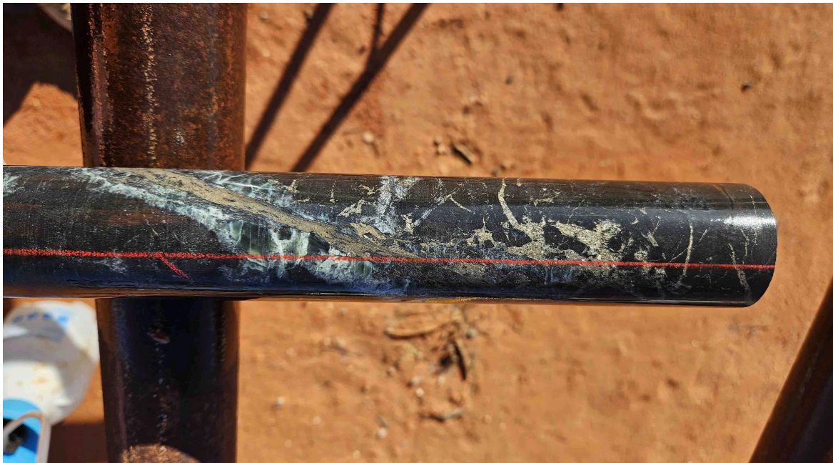
Figure 4: Example of structural vein sulphide hole MTD027
