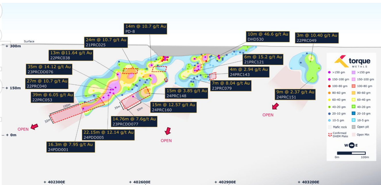
Figure 1: Paris deposit EM conductor plates modelled from DHEM surveys vectoring extensions of gold-associated sulphide minerals. Note recently surveyed holes show strong correlation between DHEM conductors and previously identified high grade gold mineralisation.
