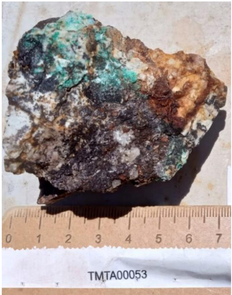
Figure 5: Toro South ‘selective’ rock chip sample (wet photo) with assay grades of 21.3ppm Ag & 1.41% Cu . The sample consists of a phyllic-altered dacite with sheeted manganese oxide and Cu-oxide veins that contain chalcantite and chrysocolla. Sample Identifier: TMTA00053 located at 432482mE, 6768818mN, WGS 1984, UTM Zone 19s). See BRX ASX release from 21 February 2024 for more sample results.
