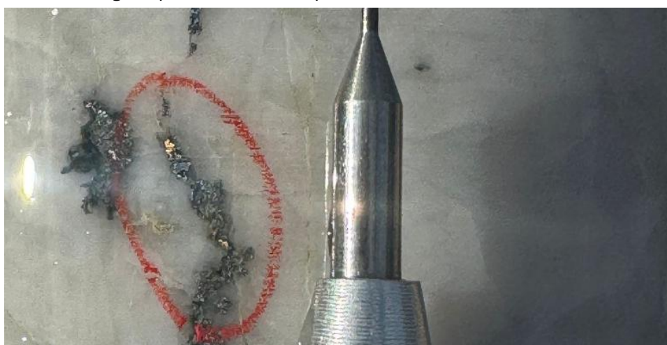
Figure 1. Diamond drill core from AMD009 at 201.6m metres down hole showing grains of visible gold 1 (yellow) to 2mm hosted in an arsenopyrite vein (grey) in milky quartz. Assays are pending for this hole.
