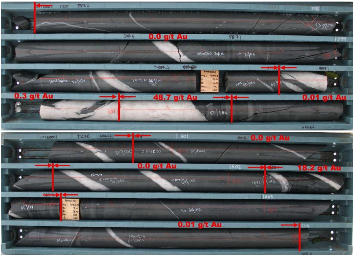
Figure 8 Photo of core trays of the mineralised zone from 600.0m to 602.4m in BMDD001
