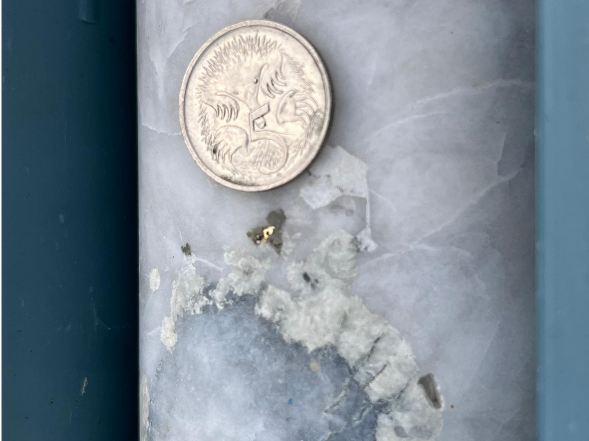
Figure 6 Visible gold at 600.2m depth associated with arsenopyrite in a quartz-carbonate vein
