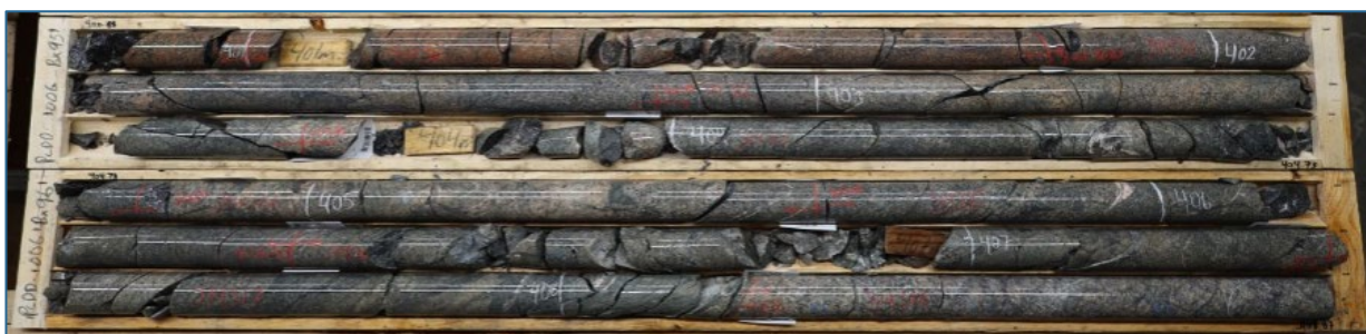
Figure 2: Example of highly anomalous hydrothermal alteration within faults and shears, PCDD006, 404.8 - 407.4m.
