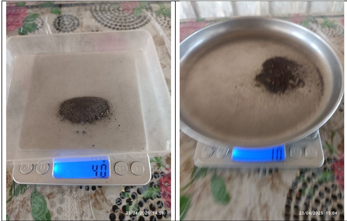
Figure 11: 4g of dried pan concentrate (Left), 1g of separated magnetic material (Right)
