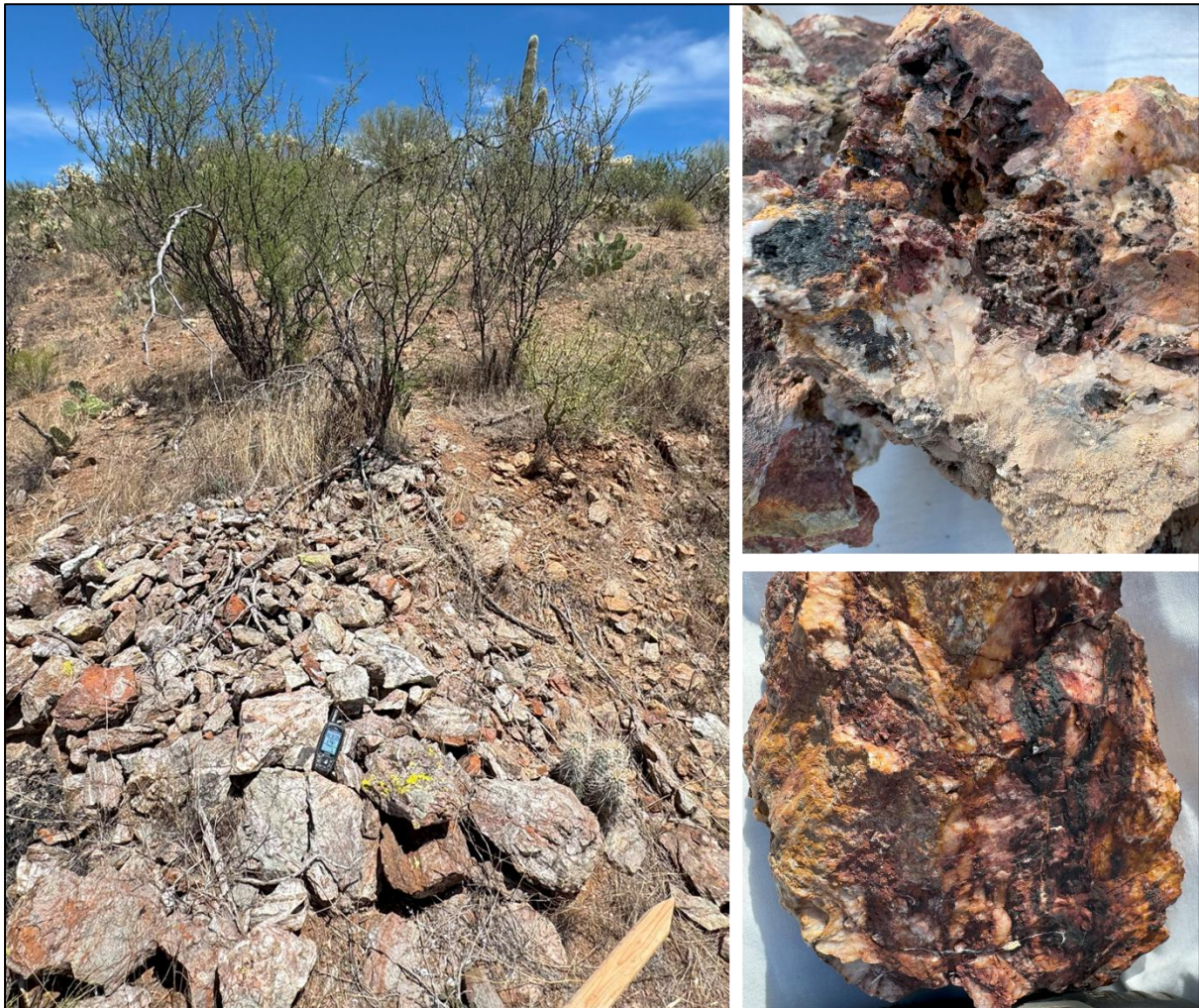
Figure 1: Aurora Prospect. Left: Sample 25RK001 29.3 g/t Au, 36 g/t Ag, 1.59% Pb. Upper right 25RK010, gossanous vein with 6.15 g/t Au, 17 g/t Ag, 1.04 % Pb. Lower right 25RK002 11.2 g/t Au, 20 g/t Ag, 0.35% Pb.
