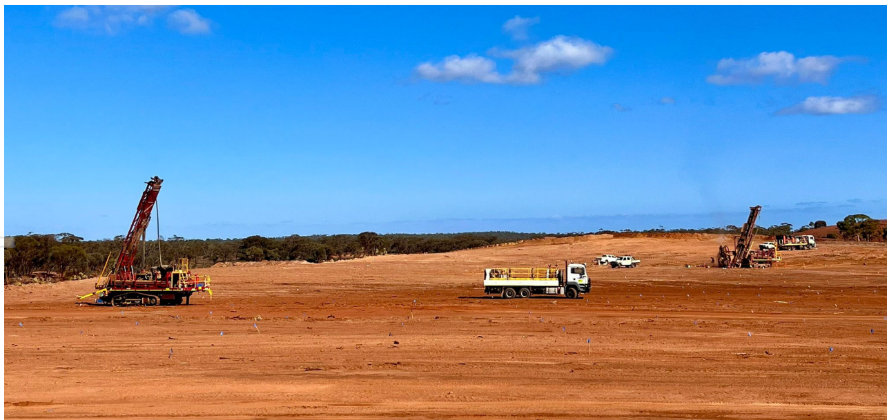
Figure 1: Grade control drilling at Fingals.
