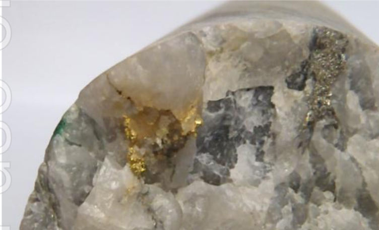
Figure 6: Visible gold identified in diamond drill hole GRC_070. Historical drill core collar GRC_070 within the Guji gold target area, referenced from the Nejo Gold Project. Source: Kefi Minerals – New Gen Gold Conference Presentation – 14 November 2017. Askari Metals has not yet verified the drilling, sampling, or assay techniques and therefore treats the information as historical and visual observations are considered qualitative and indicative only.
