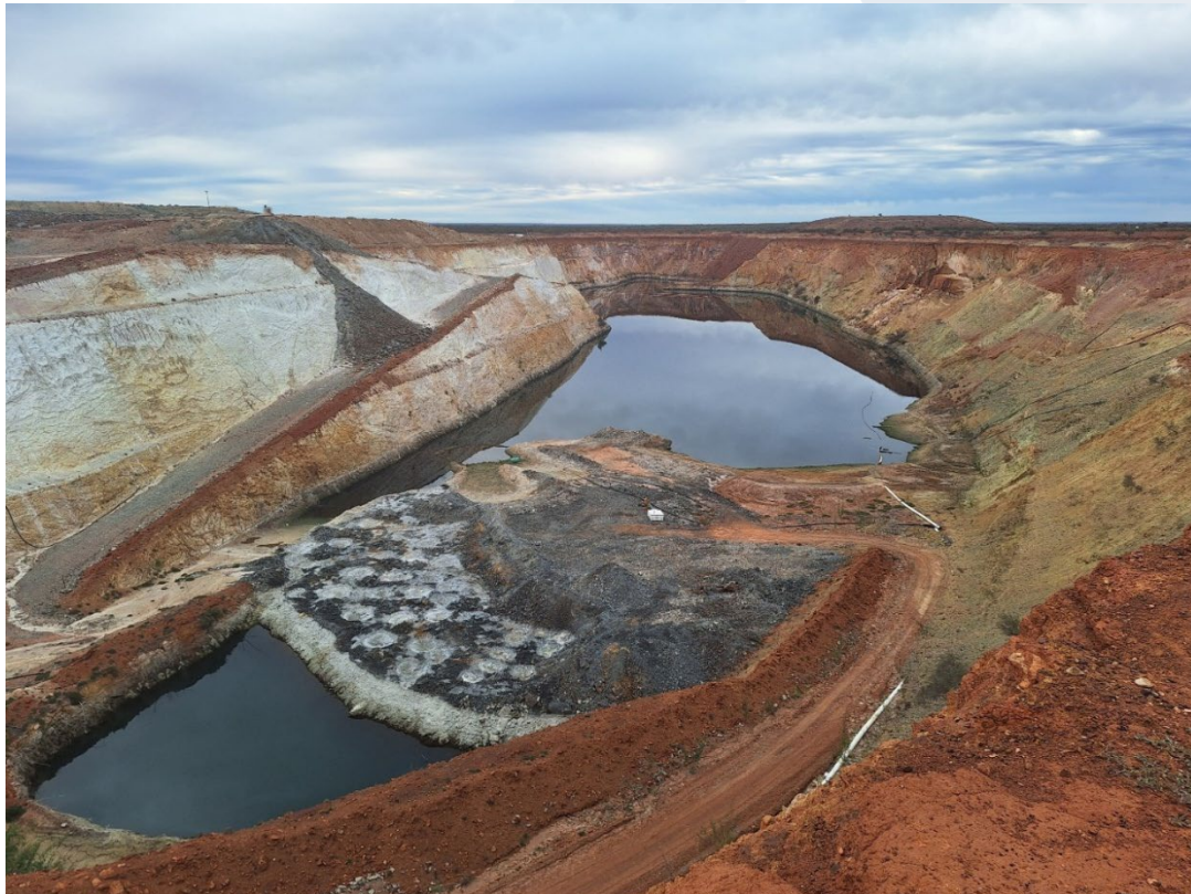
Figure 3 – Youanmi Main pit pump showing a ~3m reduction in water level
