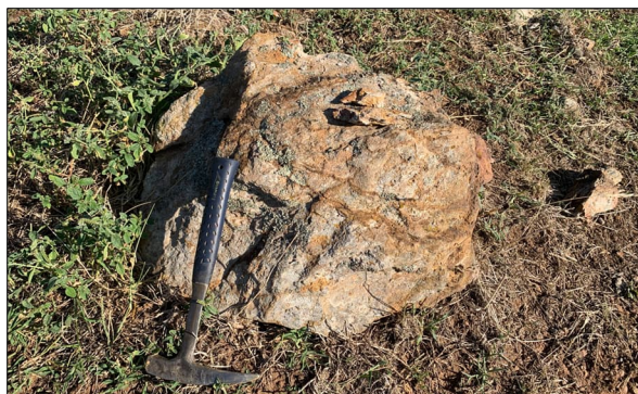
Photo 1. PWR030 (slab – left, from subcrop - right) containing disseminated limonite (after pyrite) & muscovite rich veinlets hosted in pervasive phyllic (muscovite-quartz-limonite/pyrite) altered, andesitic volcanoclastic sandstone.
