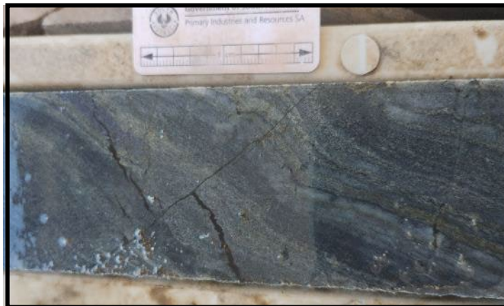
Layered to laminated, mainly Pb sulphide, recrystallised and folded, BUDD192 @ 157.7m
