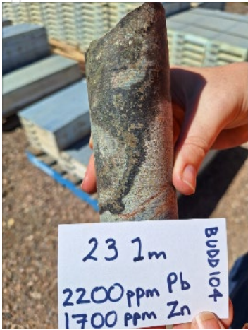
BUDD104 1 pXRF 2,200ppm Pb and 1,700ppm Zn @ 231m in sulphide vein 7m from end of hole.
