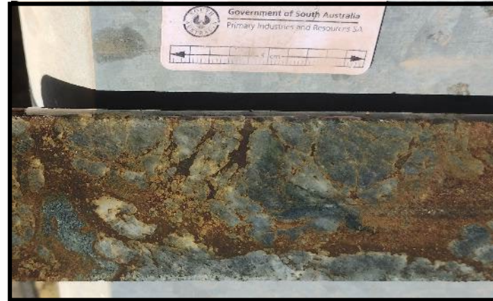
Massive pyrite/pyrrhotite often associated with milled chert/quartz vein breccia clasts, BUDD192 @ 133.6m
