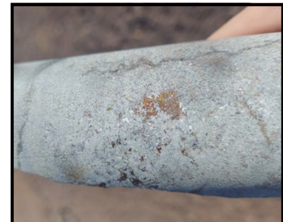
Disseminated Bornite and Sphalerite with cross-cutting veins, BUDD100 @ 451m
