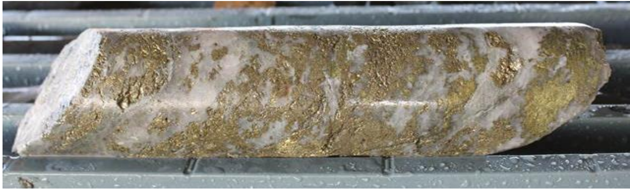
Figure 5 – The main quartz-carbonate-pyrite-chalcopyrite vein with strong sericite-chlorite selvages of the Displaced Lode mineralisation in DTDD056, grading 221.3 g/t Au, 70.2g/t Ag, & 2.71% Cu (143.5 – 143.9m).
