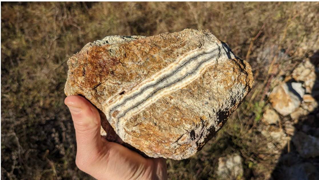
Figure 5: 2cm wide colloform-crustiform banded vein from Francis Creek comprising of quartz, adularia and marcasite (approx. 10%).
