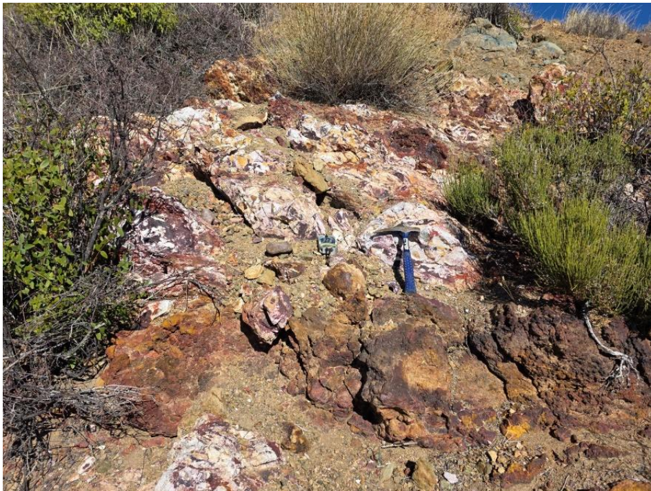
Photo 3. NW structure with abundant oxide after sulphide. Located in a low IP resistivity and moderate IP chargeability zone interpreted to be proximal to a Cu-Mo porphyry. See Figure 1 and Table 1 for location and details.
