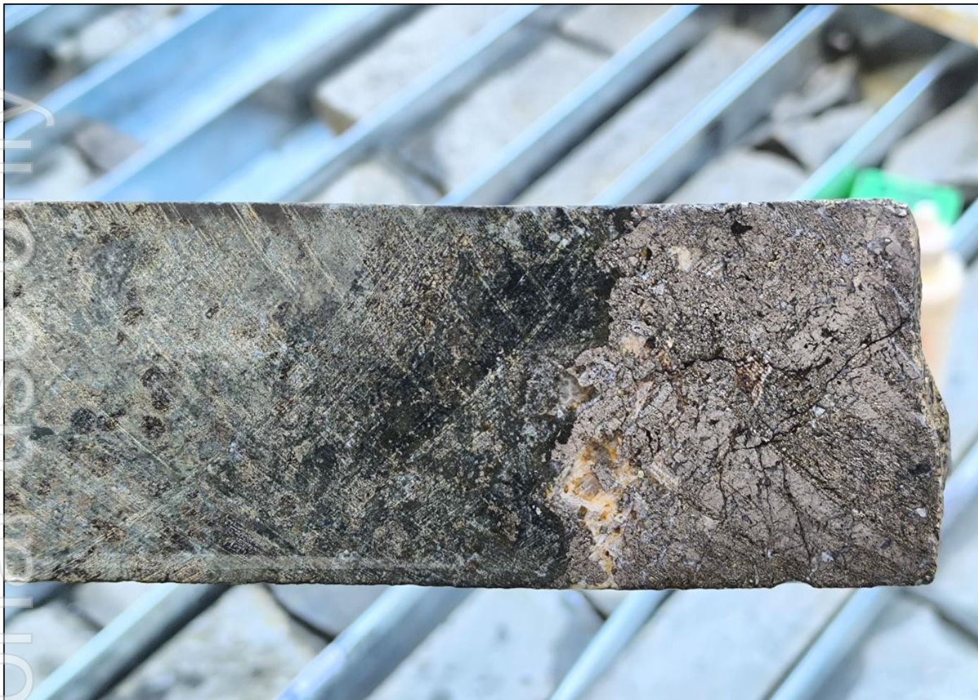
Figure 5. Core photograph from 343.1m in ZRSD25183 showing strong pyrrhotite alteration – 7.7g/t Au.
