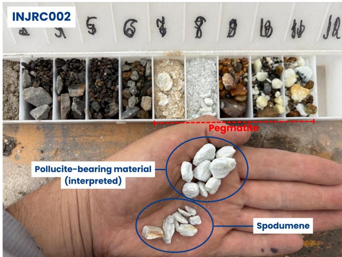
Figure 2: Downhole Samples from Hole INJRC002 at Target 1, Igrejinha Project. Drill chips and photographs are for illustrative purposes only and are not representative of the full geological interval. Geological observations are preliminary and based on visual logging. Assays are pending and should not be relied upon for grade estimation. Refer to Appendix A for rock type descriptions. No inferences regarding mineralisation or continuity should be made until certified assay results are received.
