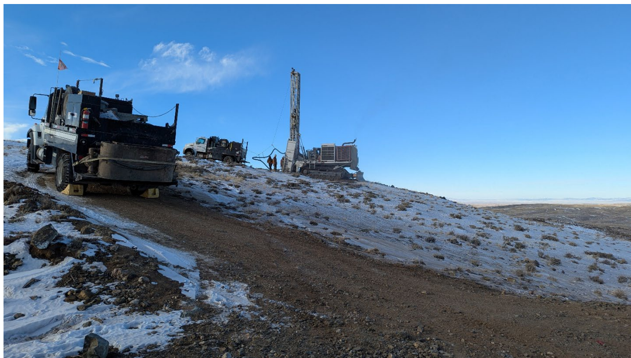
Figure 3: Boart Longyear MPD 1500 RC Drill Rig and support vehicles on site at Black Mountain.
