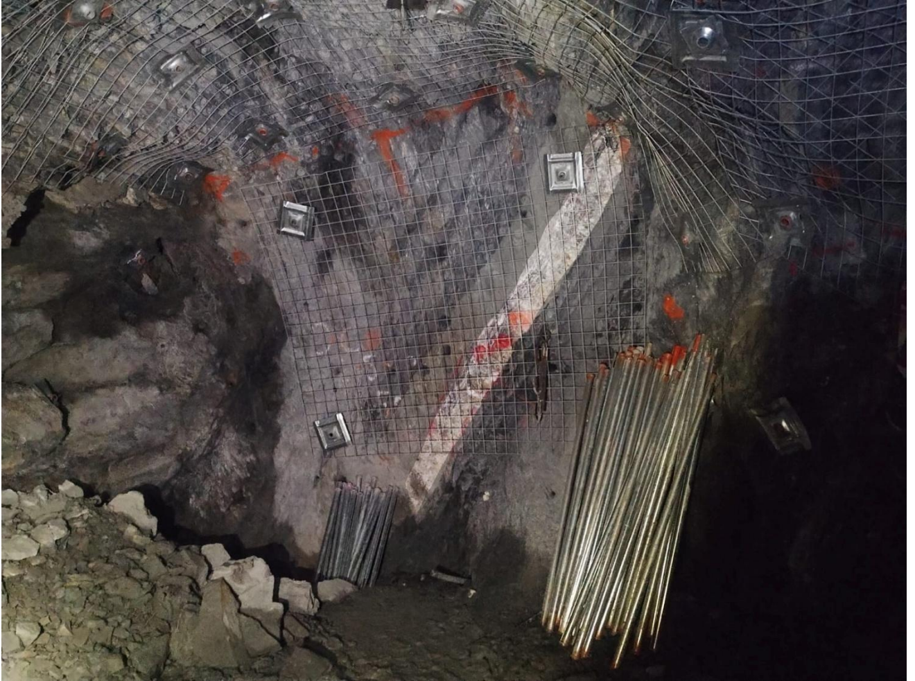
Figure 4 - The Lady Belmore quartz vein with bored out ready to charge
