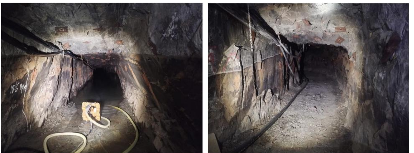
Figure 5 Mica Lense declines. One of three gold bearing declines being dewatered.
