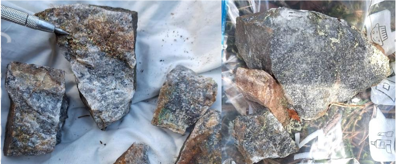
Figure 1: (left) Photograph of sample GH63 from the Domstugan Prospect of highly altered quartzite with magnetite veins showing 3% pyrite, 2.5% chalcopyrite, which assayed 1.2 g/t Au, 0.8% copper and 48 g/t Ag; (right) Photograph of sample GH68 from the Tintorp Prospect of magnetite altered quartzite and diorite with 9% pyrite, 7.5% chalcopyrite, which assayed 0.3 g/t Au, 2.2% copper.
