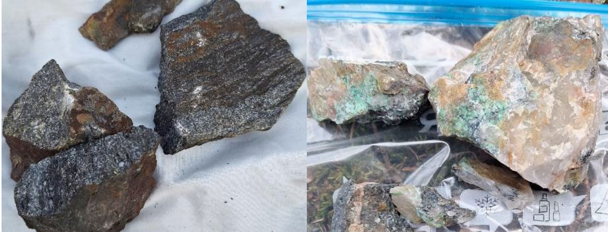
Figure 4: (left) Photo of sample GH66 from the Klubbs (Riskebo) Prospect of a quartz rich grey gneiss displaying approximately 1% fine grained pyrite, 1.5% chalcopyrite which assayed 0.6% copper and 0.05 g/t Au; (right) Photo of brecciated quartz veins with approximately 3% malachite at the Gruvdalen Prospect and assayed 1.1% Cu.
