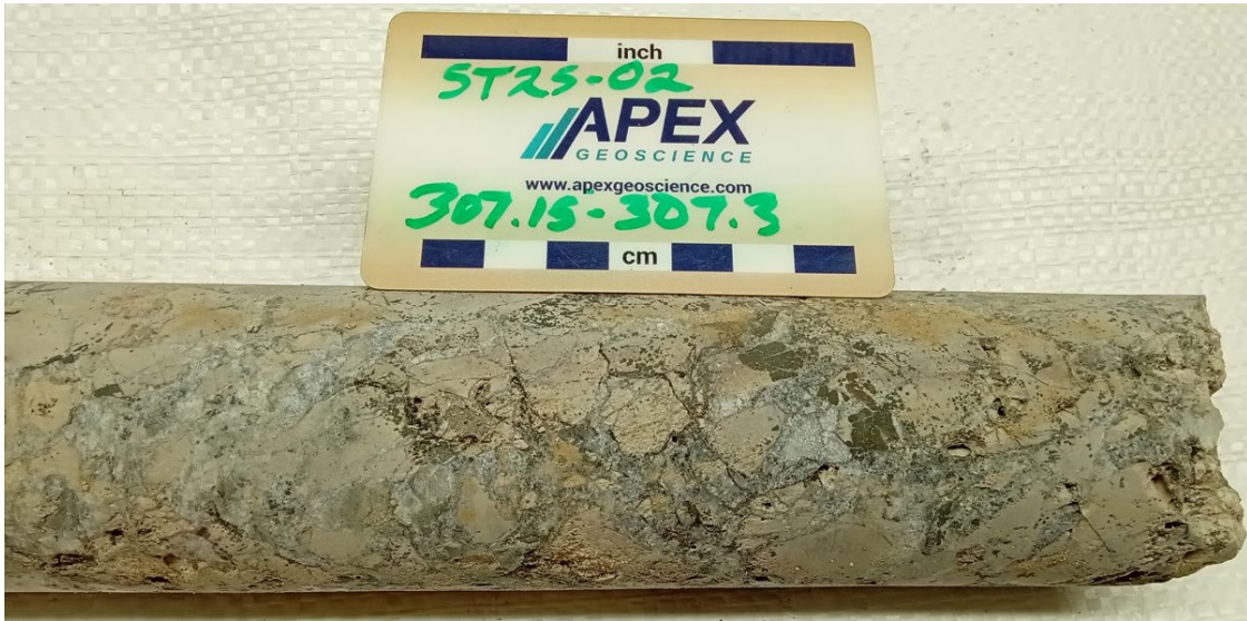
Figure 2: Dense breccia and fracture fill visual pyrite and chalcopyrite from ST25-02 (307.15-307.3m downhole). Assays for this interval are pending (see below visual estimates disclaimer).
