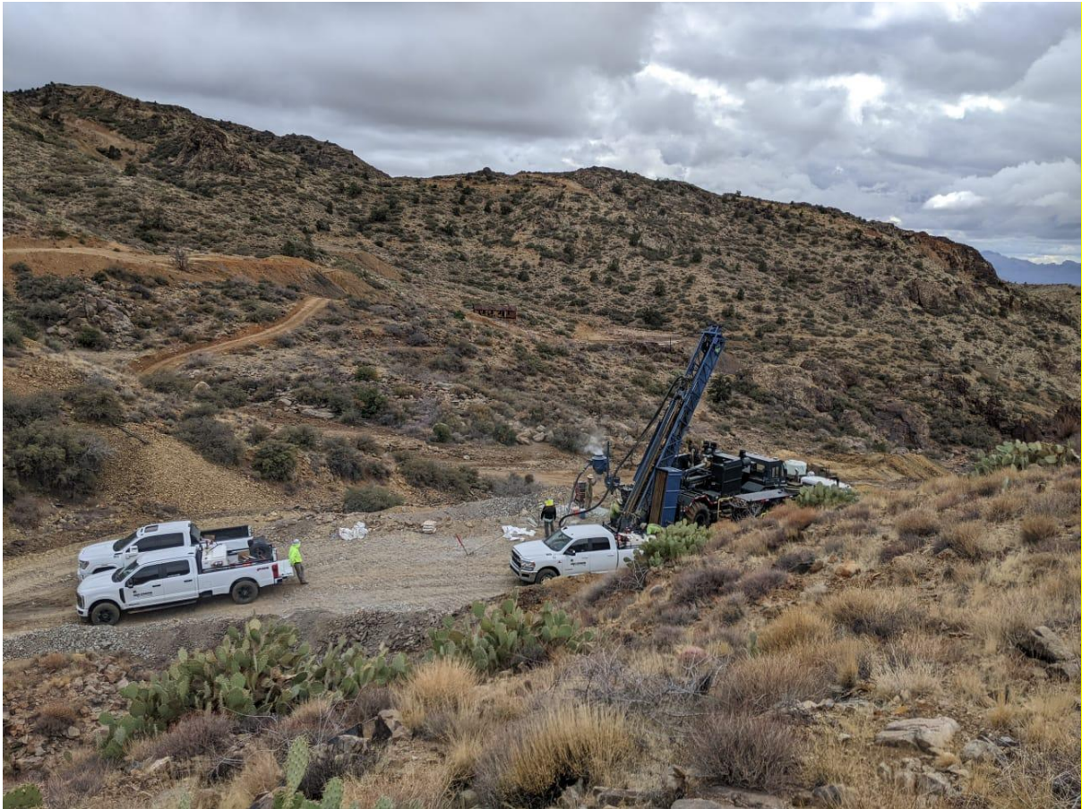
Figure 6: RC Drilling at Golconda, March 2025
