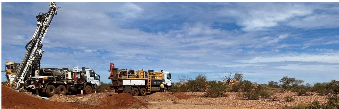
Figure 1: RC Drilling at S-Bend
